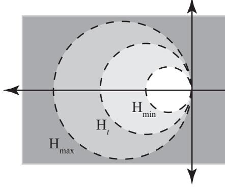
Figure 2.2: Time varying Hilger circles. The largest,  $\mathbb{H}_{\max}$  has center  $-1/\mu_{\min}$  while the smallest,  $\mathbb{H}_{\min}$  has center  $-1/\mu_{\max}$ . In general, the Hilger circle at time  $t$  is denoted by  $\mathbb{H}_t$  and has center  $1/\mu(t)$ . The exterior of each circle is shaded representing the corresponding regions of convergence (with respect to the transform).
