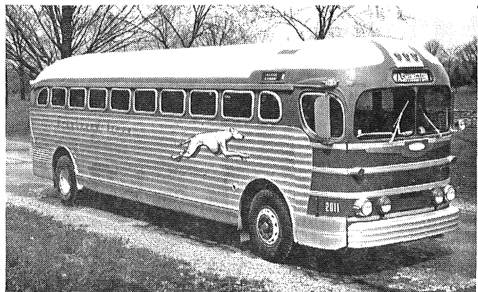
1947 General Motors (Yellow Coach name dropped) or GM PD 3751, the 51 signifying post WWII assembly. After delivery the number was changed to an Atlantic Greyhound 1800 series. This, the post war version of the famous Greyhound "Silersides" first delivered in 1941.
