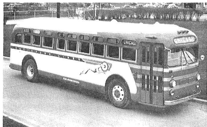
1942 Yellow Coach model TD 3605, 36 passengers, #1017. this is a transit body with standee windows, side facing seats over front wheels and small parcel racks above standee windows. Used in suburban service out of Charleston, WV.
