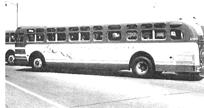
1949 General Motors model TDM 4509, T for transit, D for Diesel and M for manual transmission. 41 passengers, again with standee windows, small parcel racks but with all forward facing high seats. Again used in the Charleston area.
