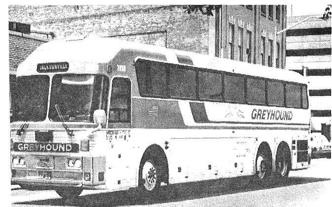
1986 MCI model 96A3 (96"-A, 1st in series, 3-axes), 47 passengers and 1988 Eagle model 15. (Delivered new to Greyhound)
